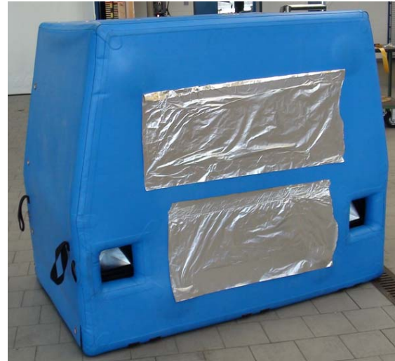
Figure 8: corner reflectors and reflexion foil on the balloon car
