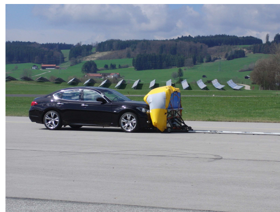
Figure 9: impact of the target in scenario leading vehicle slower
