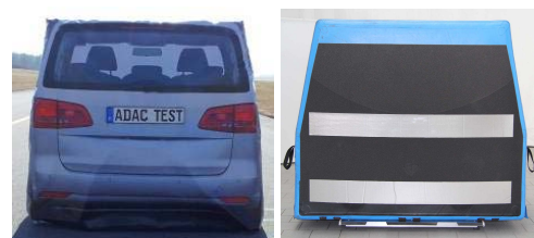
Figure 12: ADAC Target Version 3 stripped down
