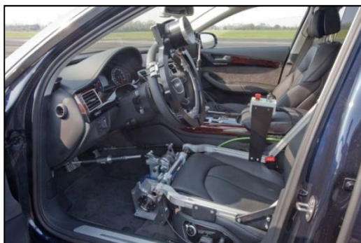
Figure 3. Combined Brake and Accelerator robot (CBAR) and steering robot used to control the test vehicle.
