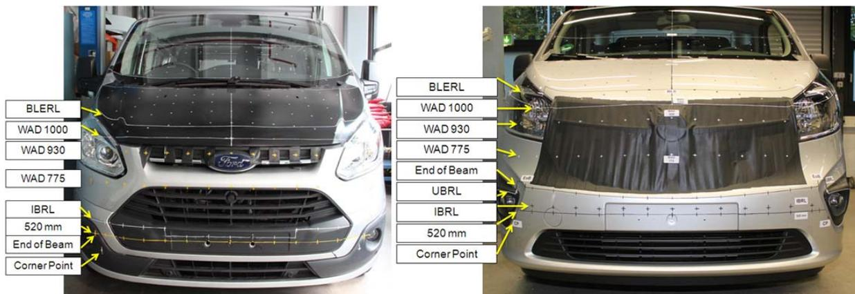
**Figure 7. Investigation on the applicability of pedestrian testing protocol to heavy vehicles.**
