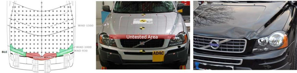
*Figure 5. Untested critical area after introduction of Euro NCAP New Upper Legform grid procedure.*
