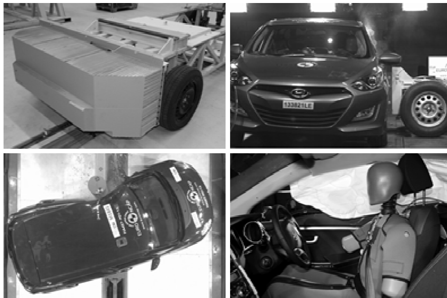
Figure 1. In 2015, the Euro NCAP side impact crash tests will be updated with new elements such as the Advanced European Mobile Deformable Barrier (AE-MDB) [3] and the WorldSID mid-sized male dummy.
