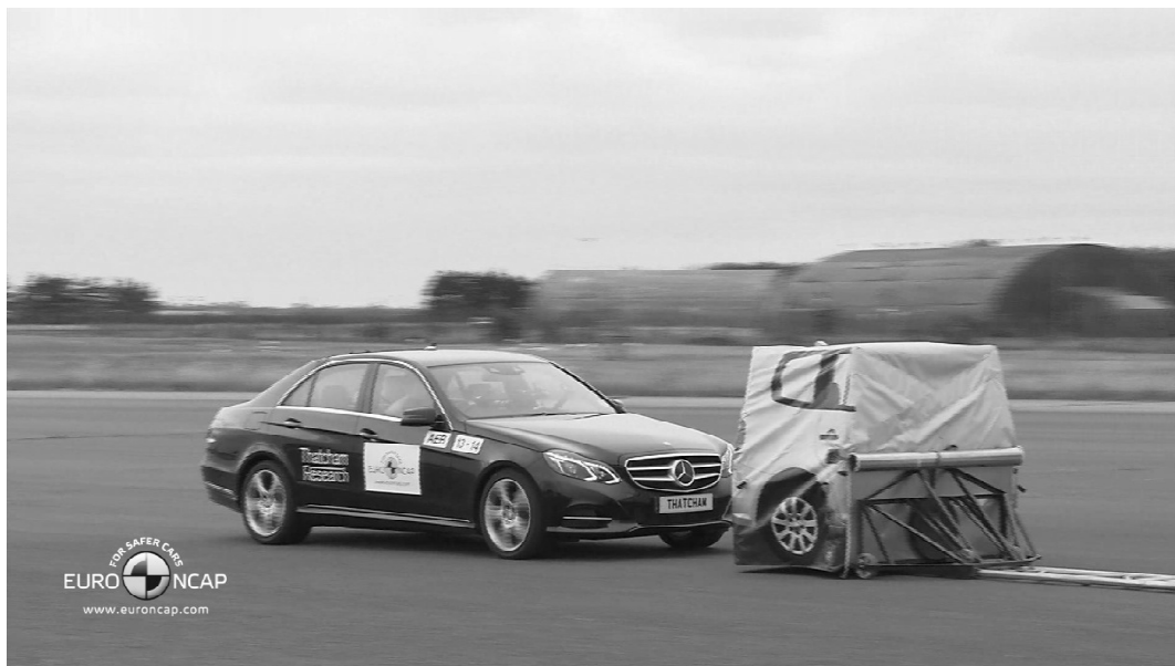
Figure 4. Euro NCAP started to assess AEB systems in 2014 using specially designed “impactable” vehicle target and test equipment.
