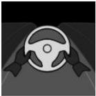
Steering wheel symbol yellow: Hands are not around the steering wheel. System remains active.
